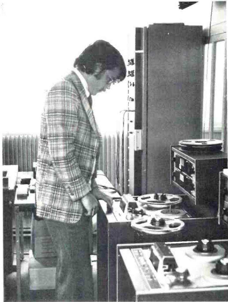
Serge Doubine starts up an ElectroSound recorder that features a third-reel capability for editing.
