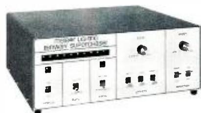
A ten channel, 1000-watt-per-channel, solid-state sequential switching device which is sound-triggered or operator-managed by an adjustable speed control.
