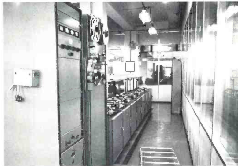
This view, taken at Pathé-Marconi, shows one of the duplicator lines using ElectroSound equipment.
